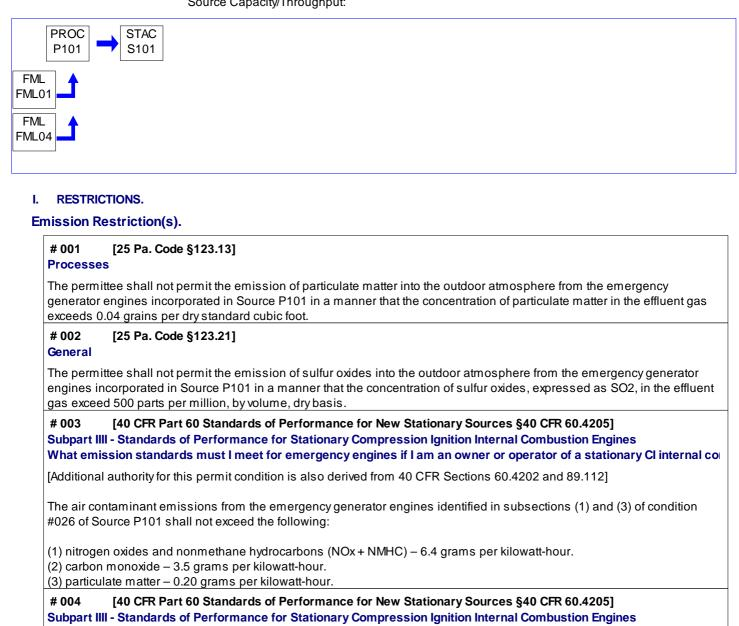
What emission standards must I meet for emergency engines if I am an owner or operator of a stationary CI internal col
